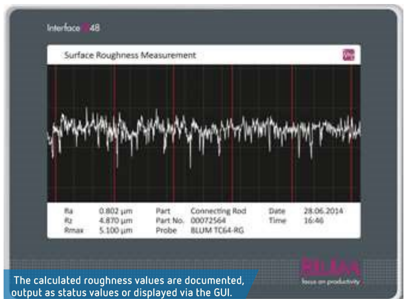
Using the special measurement insert, BLUM's TC64-RG detects surface roughness in mere seconds with \mu\text{m} precision.
